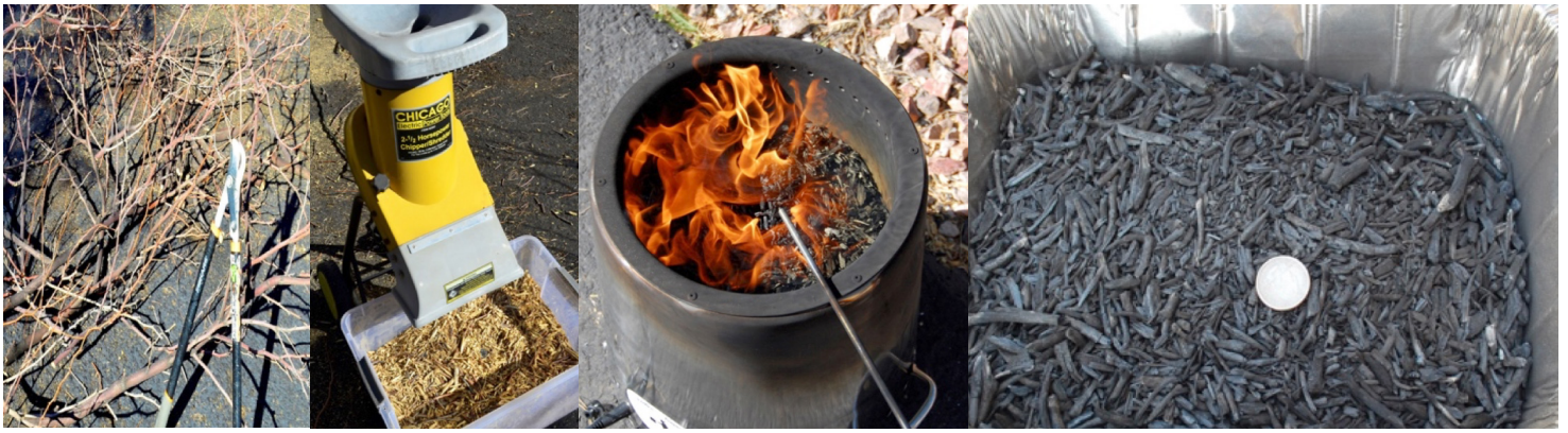
Figure 10. Mesquite Yard Waste (left), Wood Chipper (center-left), Woodgas Gasifier Stove© (center-right, no endorsement implied), Biochar (right). Photos: J. Artiola
