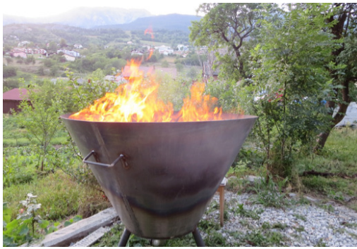
Figure 8. Japanese kiln (left). Source: www.ithaka-journal.net/86 . Biochar is produced in the pyrolysis zone where less air is available (center). Source: Image by L. Wardell. Cone with coals -- wood layer is added when the top layer begins to coat with ash (right). Source: www.ithaka-journal.net/86
