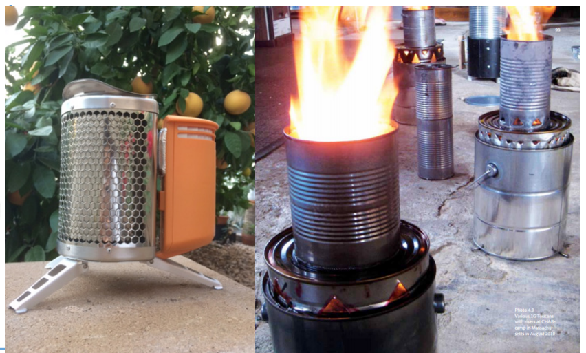
Figure 9. Basics of a Top-Lit Updraft Gasifier stove good for cooking and/or making biochar (left). Source: www.biochar-international.org . One of many types and sizes of camp stoves (center, no endorsement implied). Photo: L. Wardell. Instructions to make one are easily found online. Sizes range from coffee cans (right) to 55-gallon drums. Source: https://energypedia.info/wiki/File:Micro_Gasification_2.0_Cooking_with_gas_from_dry_biomass.pdf
