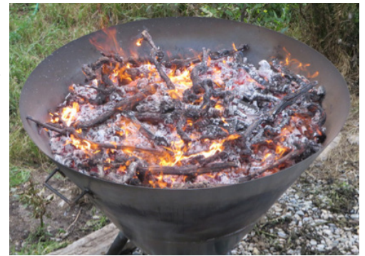
Figure 8. Japanese kiln (left). Source: www.ithaka-journal.net/86 . Biochar is produced in the pyrolysis zone where less air is available (center). Source: Image by L. Wardell. Cone with coals -- wood layer is added when the top layer begins to coat with ash (right). Source: www.ithaka-journal.net/86
